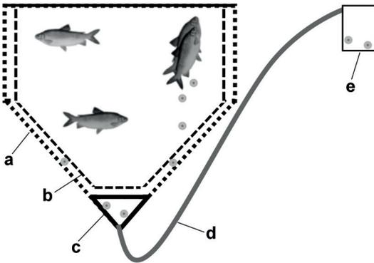
**Fig. 2.** Side-view of a cage-type device for collecting whitefish eggs during natural spawning in the absence of flow: (a) outer cage made of fine-mesh synthetic material, (b) inner cage, (c) pyramidal metal tip with a pipe, (d) hose, and (e) container for collecting eggs.
