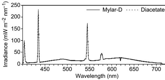
**Fig. 3.** Spectra of visible light under cellulose diacetate and Mylar-D foil. The spectra are almost identical so the spectrum under diacetate foil can be seen only in a few places.
