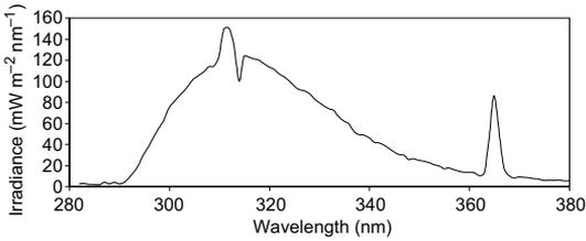
**Fig. 1.** Spectrum of UV-B lamp measured under cellulose diacetate foil.
