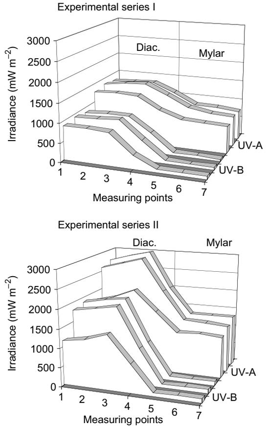
**Fig. 2.** Unweighted UV-A and UV-B irradiances in different measuring points in test aquarium in experimental series I and II. Three longitudinal measuring grids (left, middle, right) were used. The distance between single measuring points (1–7) in each grid was 10 cm.
